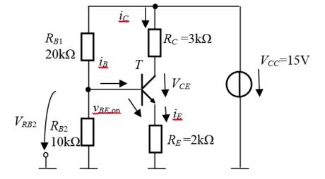
$V_{RB2}$  – obtained from the voltage divider between  $R_{B1}$  and  $R_{B2}$ , out of  $V_{CC}$
