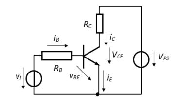
• extreme conduction or saturation (exc), BJT - closed switch:
