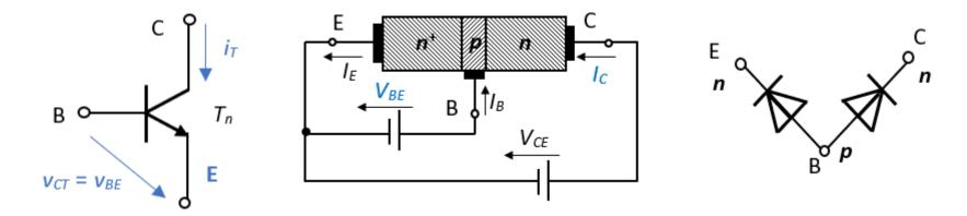
The transistor effect consists in a current flowing through a *reverse biased junction* (B-C) due to its interaction with a *forward biased junction* (B-E), placed in its very close vicinity.
