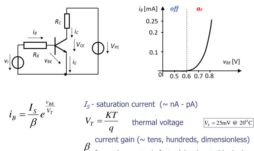
forward current gain factor (also denoted  $h_{FE}$  in dc or  $h_{fe}$  in ac)
