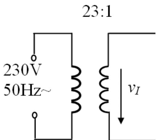
$$\widehat{V}_I = \frac{\widehat{V}_S}{n}, \text{ n-transformer ratio}$$
