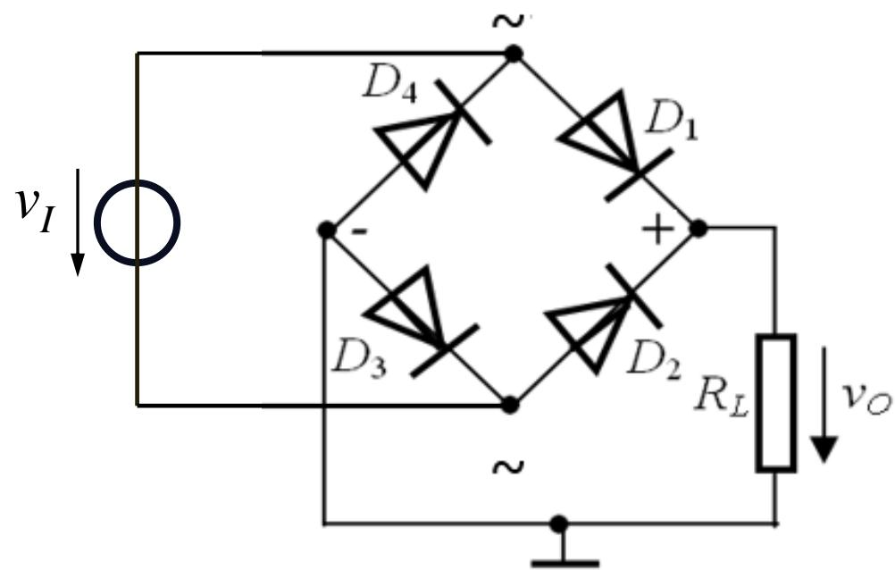
For the circuit in the figure,  $R_L = 50 \Omega$ . Assume  $\hat{V}_I = 5 \text{ V}$ .
