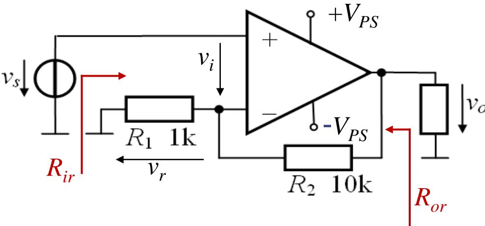
$$R_{ir} = R_i(1 + ar) = 36.4 G\Omega$$
