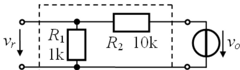
$$r = \frac{v_r}{v_o} = \frac{R_1}{R_1 + R_2} = \frac{1}{1 + 10} \approx 0.091$$
