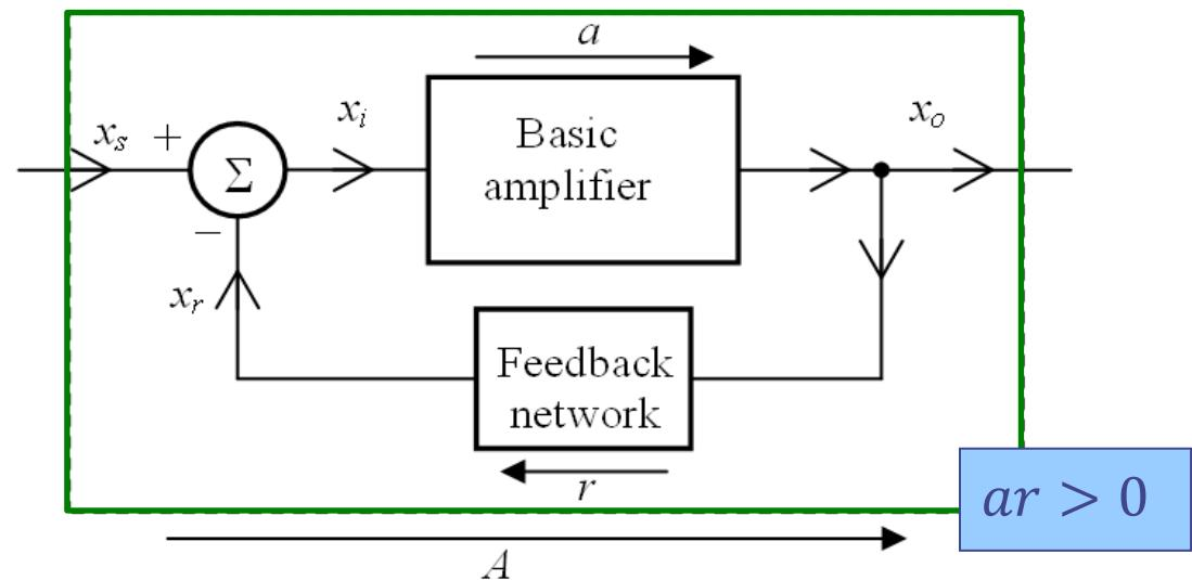
How can  $A$  be computed, using  $a$  and  $r$ ?
