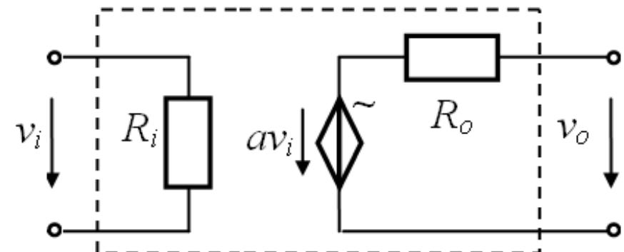
Equivalent model of the feedback amplifier
