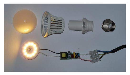
Disassembled LED-light bulb with driver circuit board (dc power supply) E27 base, 5W, 450lm, CRI >7
