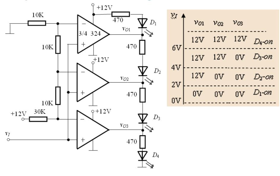
Design a bar graph optical indicator for the voltage level using 5 LEDs
