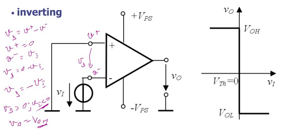
How does the output voltage look like if the input voltage is a sine wave with 3V amplitude and the supply is  $\pm V_{PS} = \pm 12 \text{ V}$ ?
