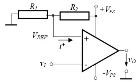
$i^+ << \text{current through}$  $R_1, R_2 \text{ divider } (i^+ \cong 0)$
