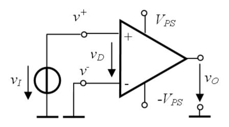
$$v_{\mathcal{O}} = \begin{cases} V_{\mathcal{O}H} & \text{if } v_{\mathcal{D}} > 0, \text{ this is } v_{\mathcal{I}} > 0 \\ V_{\mathcal{O}L} & \text{if } v_{\mathcal{D}} < 0, \text{ this is } v_{\mathcal{I}} < 0 \end{cases}$$
