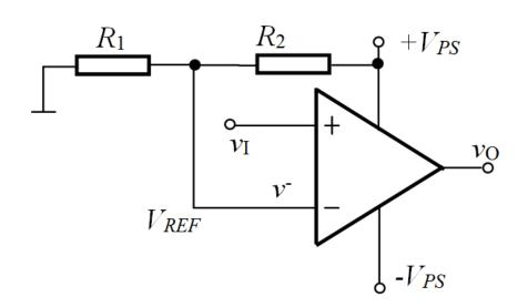
$$V_{REF} = \frac{R_1}{R_1 + R_2} V_{PS}$$
