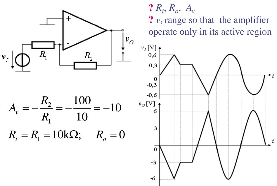
**Design example** Design an inverting amplifier with  $R_i > 8K$ and  $|A_v|$  adjustable in the range of [10,18]
