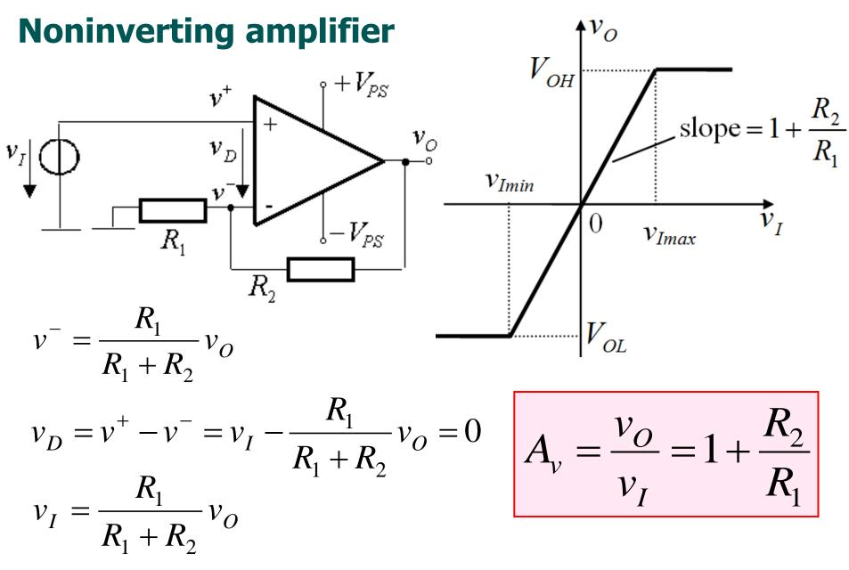
In a non-inverting amplifier, the output voltage changes in the same direction as the input voltage.
