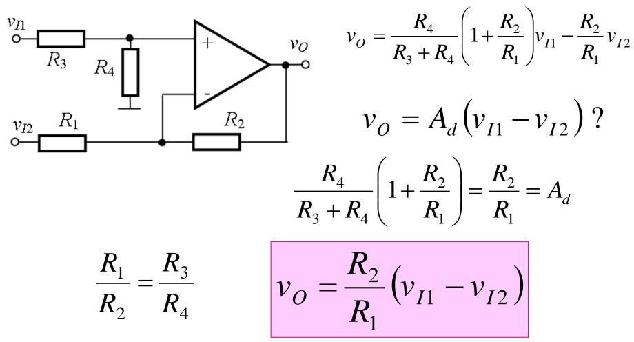
for  $v_{I1} = v_{I2}$  results  $v_O = 0$ ,
