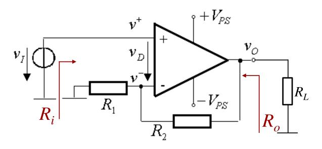
$R_i$  the resistance seen by the input voltage source
