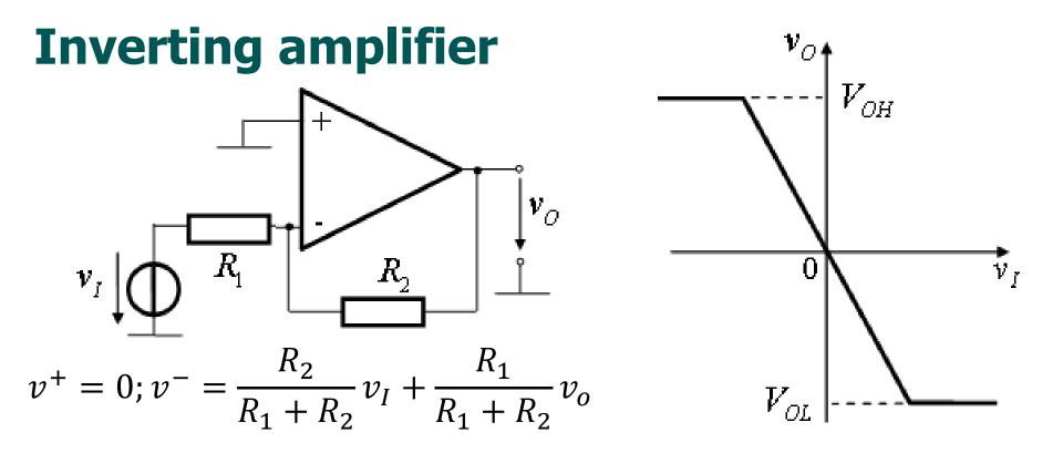
$$v_D = v^+ - v^- = 0 - \frac{R_2}{R_1 + R_2} v_I - \frac{R_1}{R_1 + R_2} v_o = 0$$
