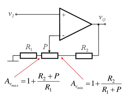
$$A_{v} \in \left[1 + \frac{R_{2} + P}{R_{1}}; 1 + \frac{R_{2}}{R_{1} + P}\right]$$
