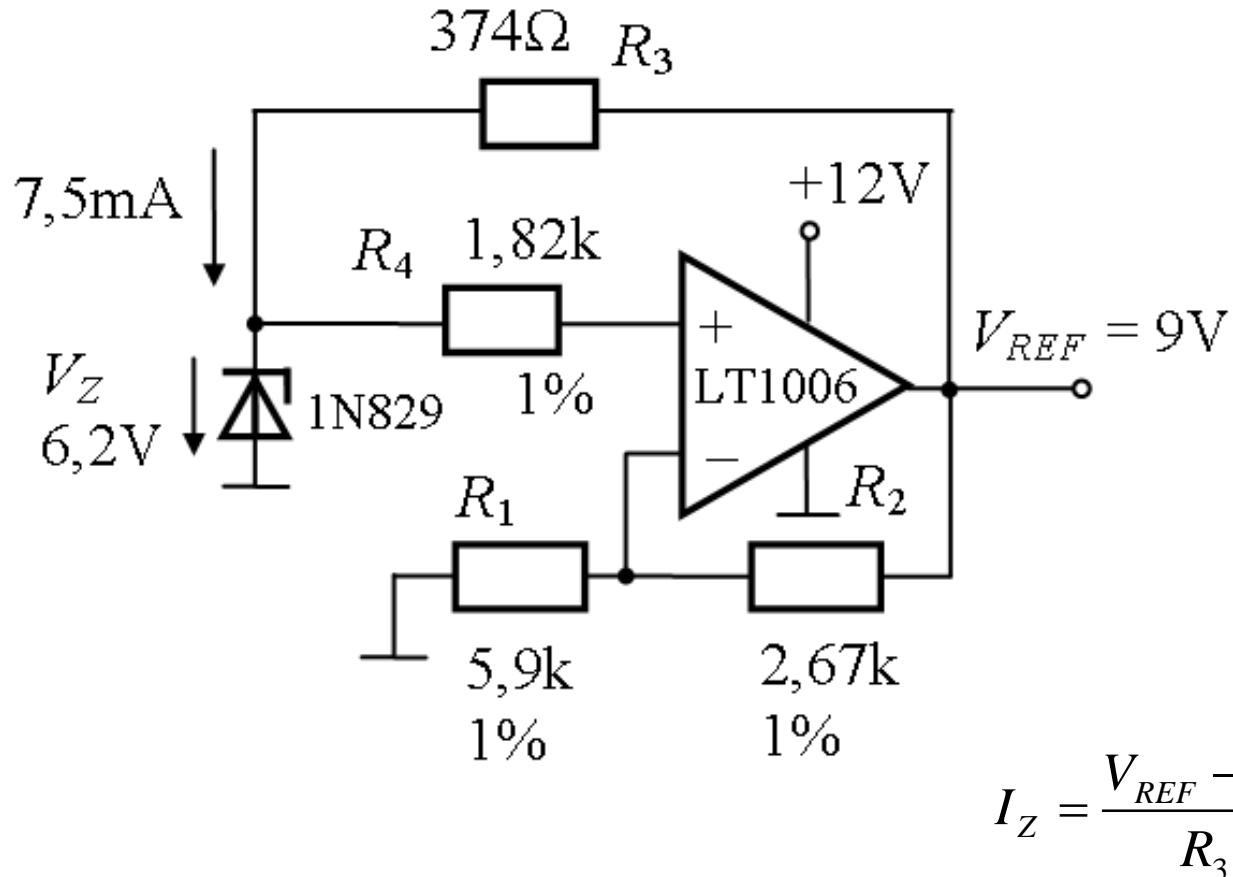
$$I_Z = \frac{V_{REF} - V_Z}{R_3} = \frac{9 - 6.3}{374} = 7.5\text{mA}$$
