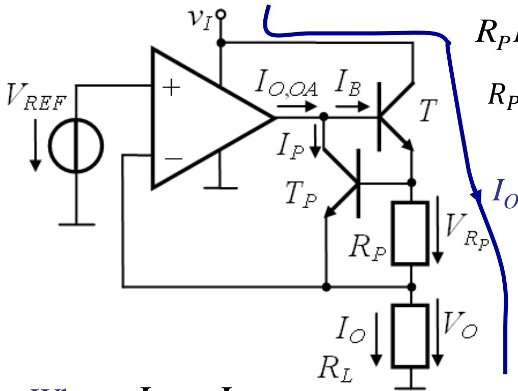
$$R_P I_O < 0.6V; \quad T_P - (off); \quad I_P = 0$$
