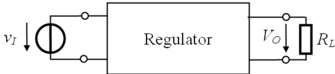
$$V_O = v_I - v_{\text{regulator}}$$
