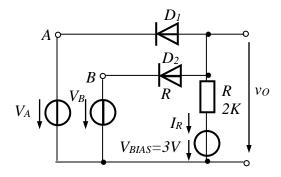
these voltage levels and give the logic table of the circuit with inputs A, B and output Y.
